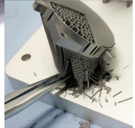
Mechanical removal of support structure after thermal treatment
