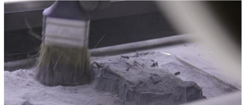
Mechanical removal of powder after AM build process
