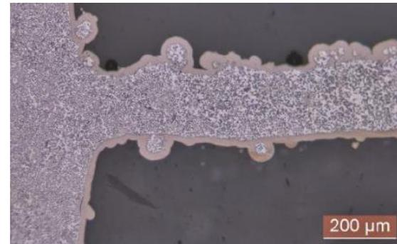
Cross-sectional view of exemplarily part with NiP plating on internal structure
