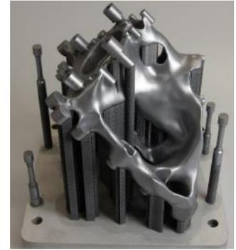
FEM simulation of topology optimized housing (left) and housing after AM build process (right)
