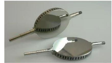
CT scan of internal mirror structure (left) and mirrors after machining (right)
