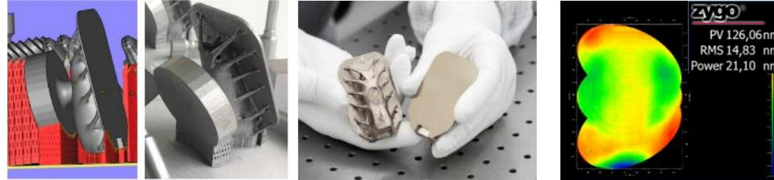
Scan mirror (left: during AM process preparation, middle left: after AM build process, middle right: after final processing incl. diamond turning, NiP plating and polishing, right: final shape deviation after MRF polishing)
