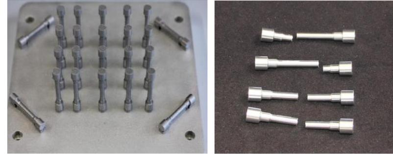
Tensile test specimens on AM build plate
