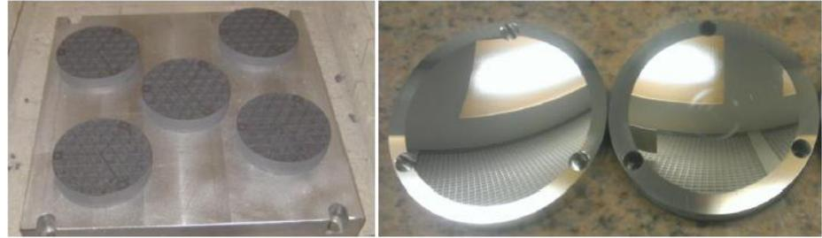
Left: batch light-weighted isogrid test mirror (AlSi10Mg, Ø 75 mm, EOS machine)
