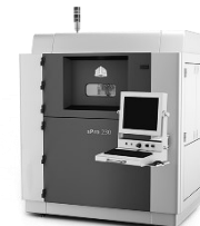
3D-Systems sPro230 ( CO 2 Laser ) 550 x 550 x 750 mm 3 PA12
