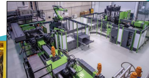
Hot forming and functionalization in the hybrid injection molding process
