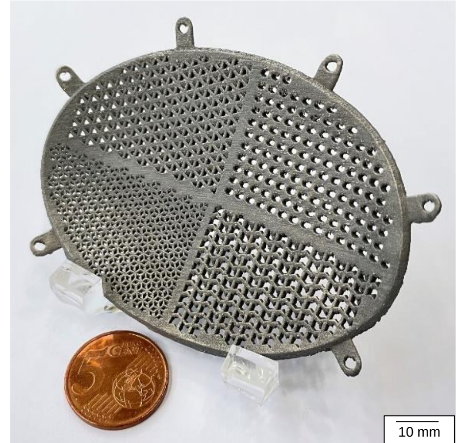
Cranial implant lattice demonstrator
