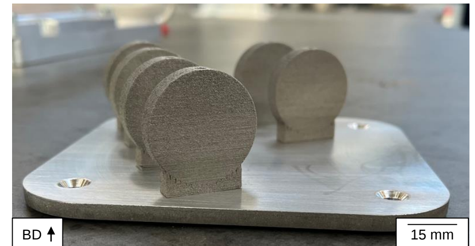
As-built hollow cylinders. Crack-free appearance after PBF
