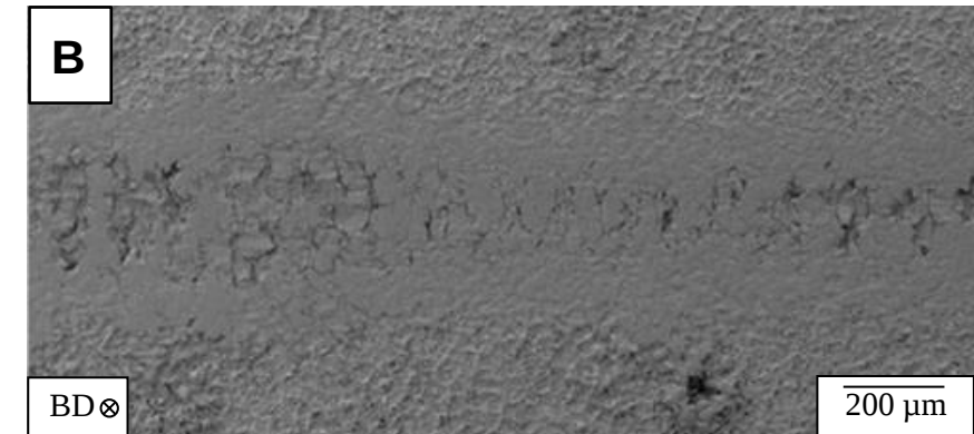
A: Progression of COF for different load cases on different ceramic surface thicknesses; B: 40 μm Surface after high load testing
