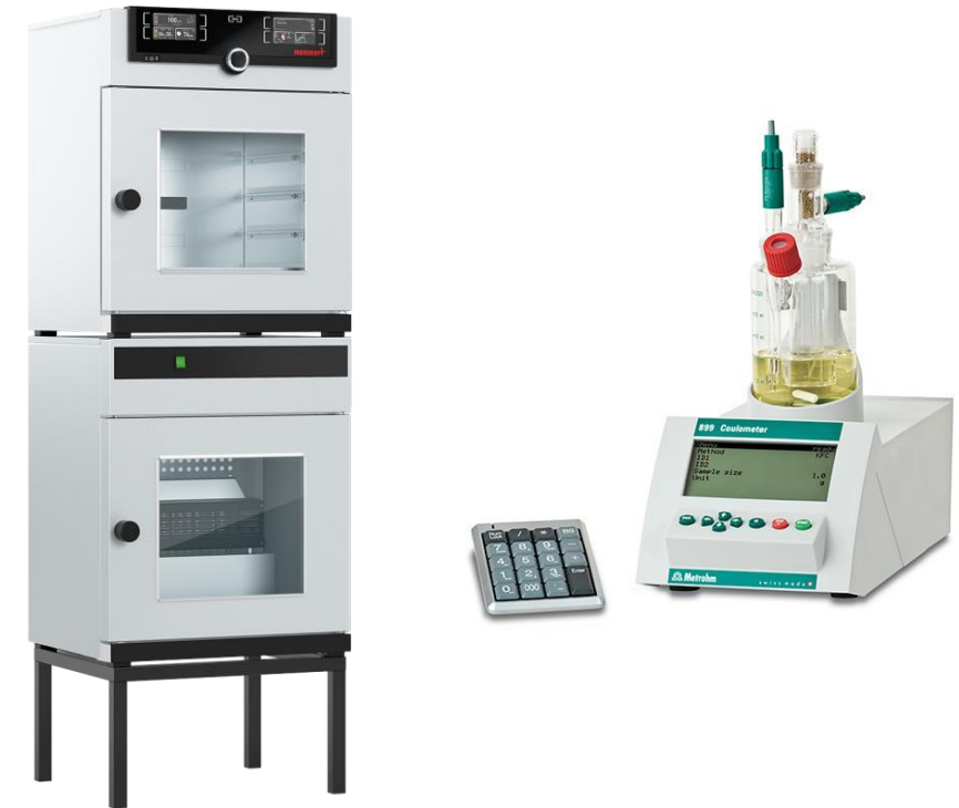
Used vacuum furnace from Memmert (VO49) as well as measuring setup for Karl Fischer titration for the determination of powder moisture
